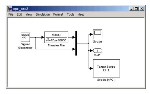
The Simulink block diagram opens for the model xpc\_osc2.md1.
