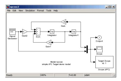
**4** To rebuild the target application, in the Simulink window and from the **Tools** menu, select **Real-Time Workshop**. From the **Real-Time Workshop** submenu, click **Build Model**.
