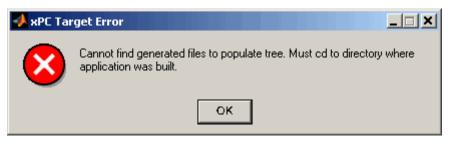
• When you built the target application, you selected the **Include model** hierarchy on the target application check box in the xPC Target Options pane.
