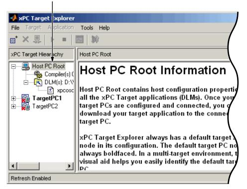
You can also start xPC Target Explorer from the Simulink model window (Tools > Real-Time Workshop > xPC Target Explorer).
