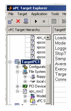
Alternatively, you can now drag a prebuilt target application, DLM, to a target PC icon. If a connection does not already exist, xPC Target Explorer optionally creates a connection to that target PC.
